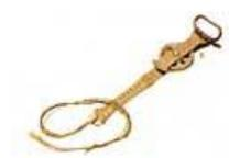
This is a pulley-like tool used to wind in the main kite-line. It is needed because the kite-lines become hot due to friction during the battles.
